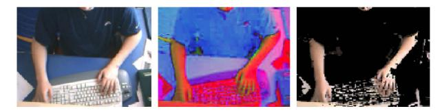
Figure 1: Skin color detection result (Raw video frame, HSV conversion of the raw video frame, Skin color filtering result)
